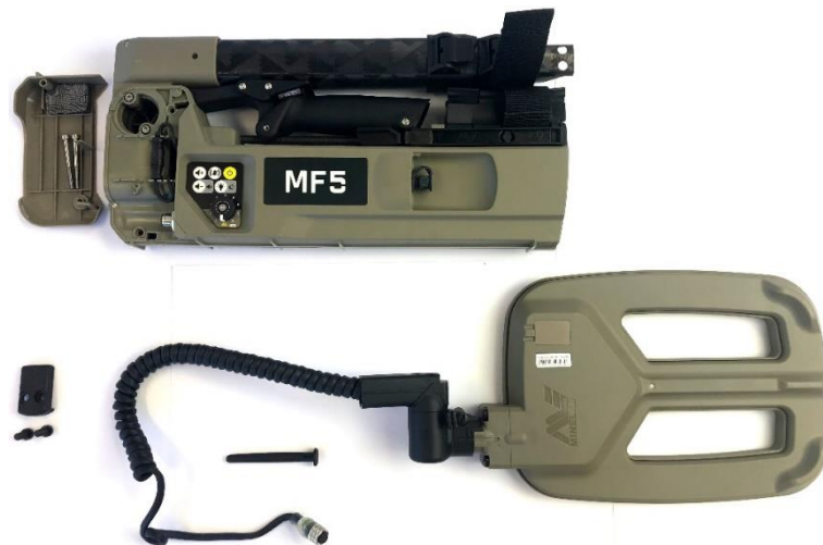
Figure 50: Coil removed from detector.
